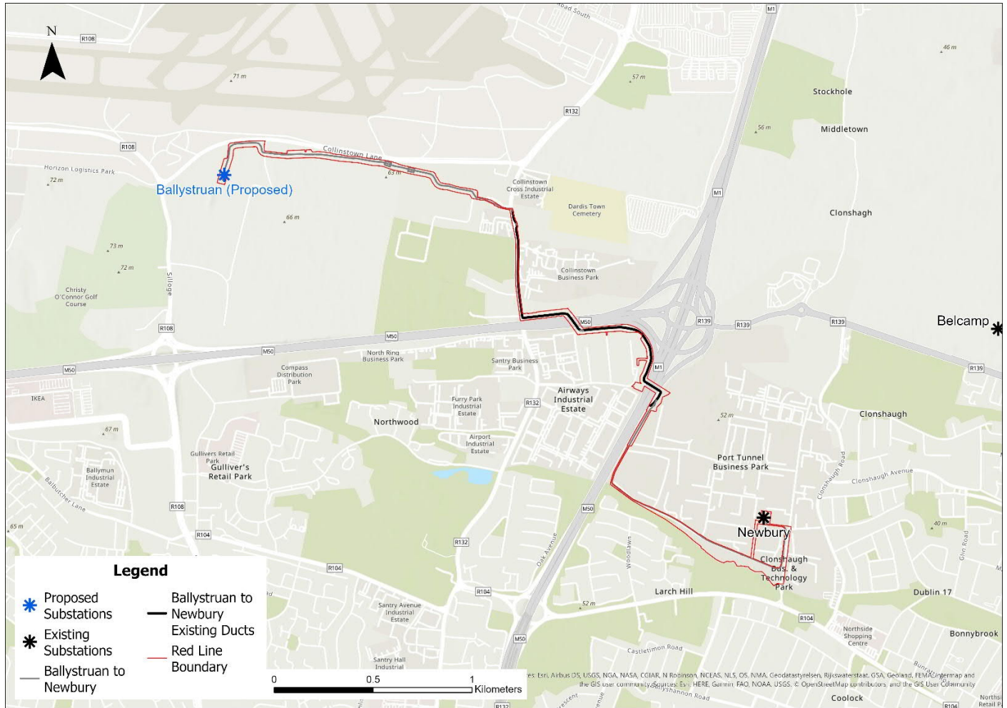
Figure 1.2: Newbury to Ballystruan 110kV UCG Route
